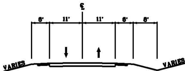
**Figure 11.3 - Cross Section for Rural Spot Improvements**
